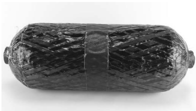
FIGURE 1. Fully infused small-scale (7.5 liter) COPV
