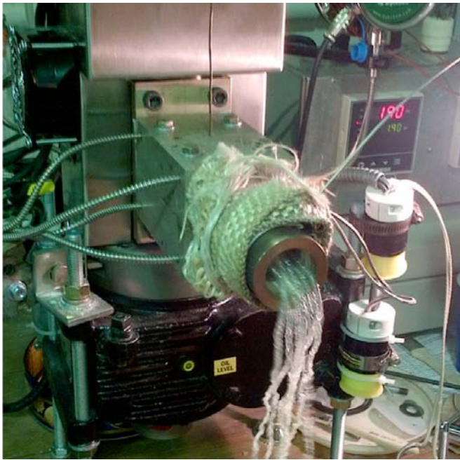
FIGURE 5. Fiber spinning using PAN pellets without the pressure chamber
