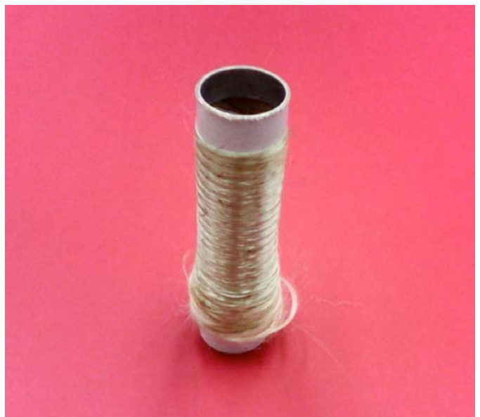
FIGURE 9. PAN filaments generated from 397-hole spinneret; the diameter of each filament is about 35 microns
