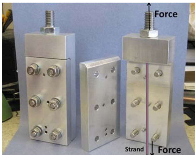
FIGURE 3. Grips selected for the stress rupture test
