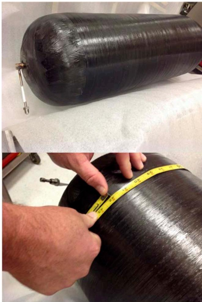
**FIGURE 1.** First thin-lined (1.8 mm) high volumetric efficiency (81%) Type 3 (metal-lined, fiber-wrapped) 700-bar experimental pressure vessel prototype
