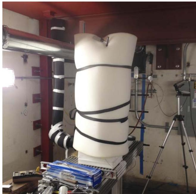
**FIGURE 2.** Cryogenic pressure test of thin-lined, high volumetric efficiency experimental pressure vessel prototype
