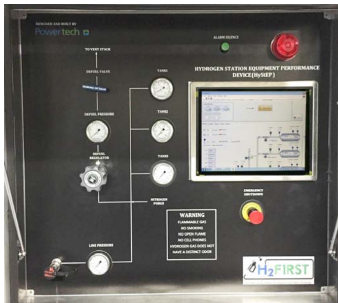
FIGURE 3. HyStEP device operator panel including receptacle, system pressure indicators, touchscreen panel, electro-static discharge, and vent controls
