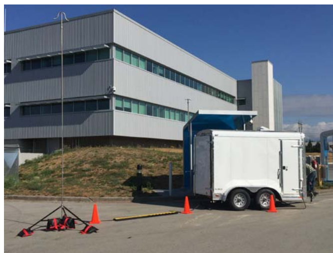
FIGURE 4. HyStEP device sited at Powertech's H 2 dispenser with the remote vent stack
