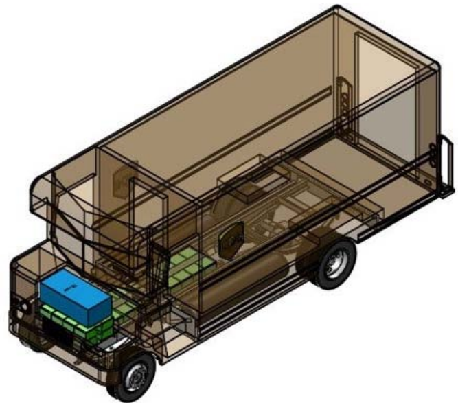
FIGURE 2. Physical layout and component packaging with van body
