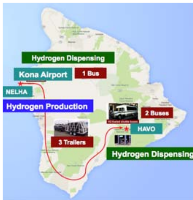
FIGURE 1. Hydrogen Production and Delivery System
