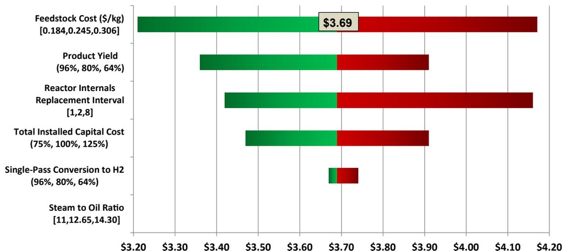
**FIGURE 3.** Tornado chart for hydrogen production via piston-type reforming reactor with pyrolysis oil feedstock. Replacement of reactor internals encompasses replacement of the monolith, catalyst, and sorbent in the reactor.
