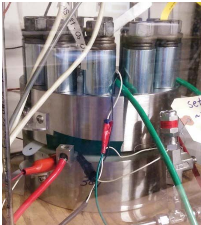
FIGURE 3. Fuel cell stack hardware designed to withstand 350 bar operational pressure
