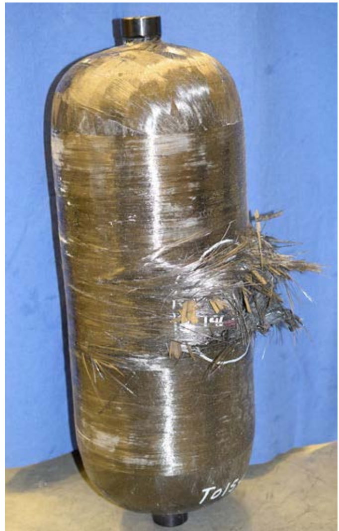
FIGURE 1. Image of burst tank made with vinyl ester resin after impact testing
