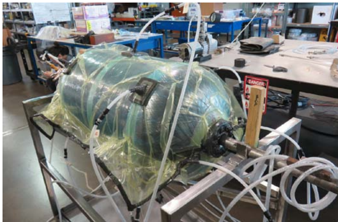
FIGURE 2. Full-scale tank (133 L) prepared for vacuum infusion
