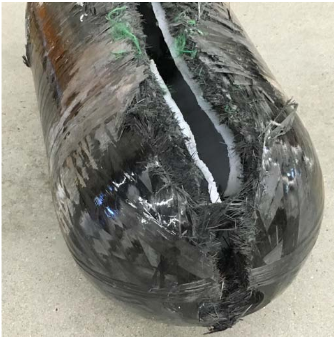
FIGURE 1. Type IV pressure vessel with Toray T700 carbon fiber after burst
