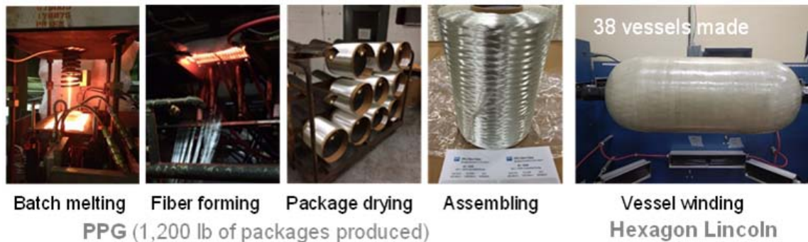
FIGURE 1. Process flow of high-strength glass fiber production, multi-end roving package assembling, and tank winding processes
