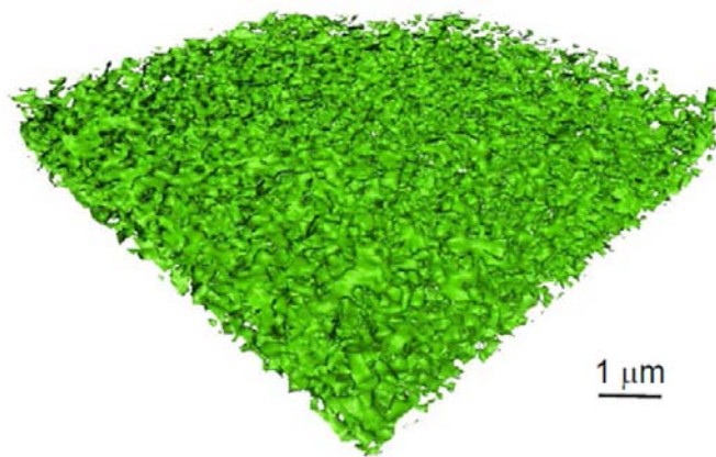
FIGURE 10. 3D imaging of ionomer dispersions in catalyst layers. Individual F maps were acquired from slices and stacked to create a 3D rendering of the ionomer distribution.
