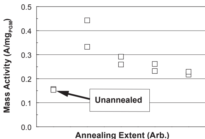
FIGURE 2. Mass activity sensitivity vs. annealing extent for single UTF “A” composition
