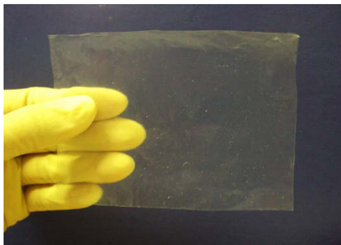
FIGURE 1. A sample membrane of the new PEM prepared at Amsen
