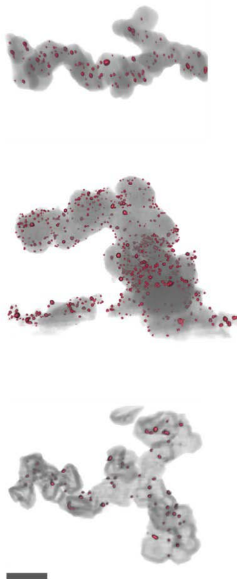
FIGURE 1. STEM electron tomography reconstructions demonstrating the location and size differences of Pt nanoparticles (loading of 5%) supported on HSAC (top image), V (middle image), and LSAC (bottom image)
