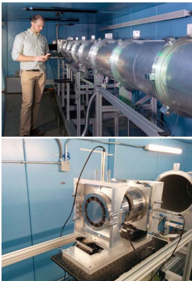
FIGURE 3. Top showing the inside the new cold neutron imaging instrument that was commissioned in August of 2015. Bottom showing the engineering test optic mounted on the beam line to test the NASA fabrication methods. Based on the analysis of the results a final 1:1 optic will be delivered to NIST for the user program in 2017.
