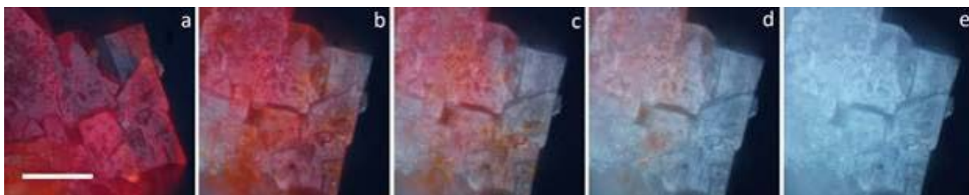
FIGURE 3. Optical micrographs of KCAT crystals exposed to H_2 gas for (a) 0 min, (b) 55 min, (c) 85 min, (d) 112 min, (e) 150 min. Scale bar = 100 \mu m.
