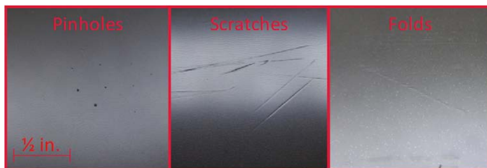
FIGURE 2. Membrane samples illustrating each of the main defect types, including pinholes, scratches, and folds taken edge-lit with a compact camera
