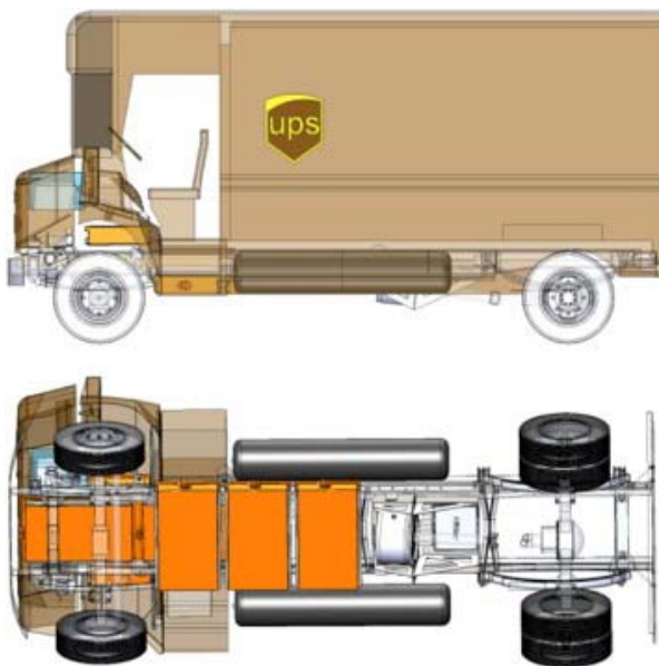
FIGURE 2. Physical layout and component packaging with van body
