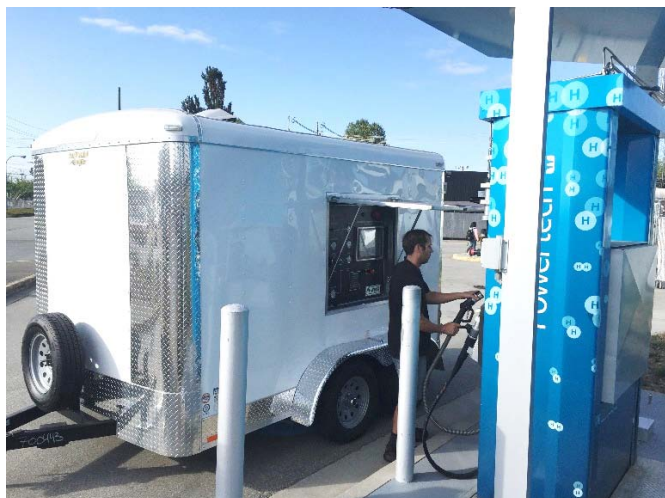
FIGURE 1. HyStEP device sited at the Powertech hydrogen dispenser
