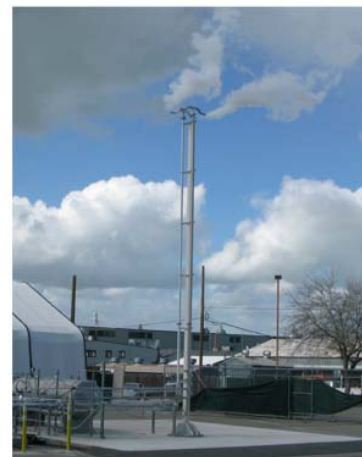
35 kg/hr, ~5 bar cryogenic H 2 release
