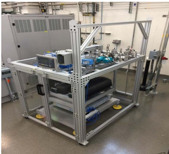
FIGURE 1. Flow meter test apparatus
