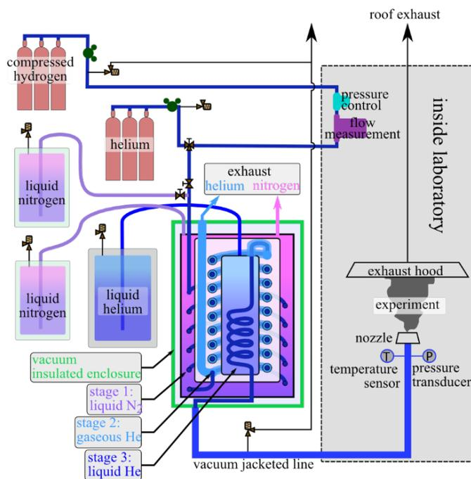
**FIGURE 1.** Sketch of the cryogenic hydrogen release experiment at the Turbulent Combustion Laboratory, Sandia National Laboratories
