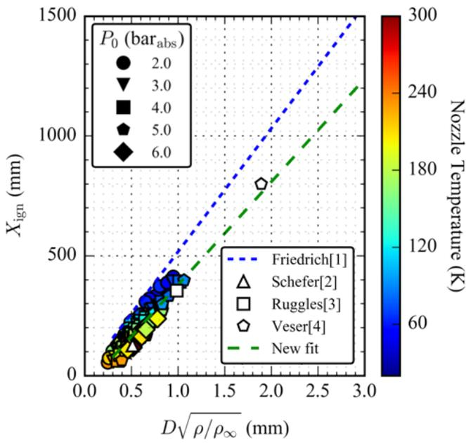
**FIGURE 2.** Maximum ignition distance as a function of effective diameter, for the cryogenic hydrogen releases in the current study and data from the literature. Blue dashed line shows a correlation from Friedrich et al. [1].
