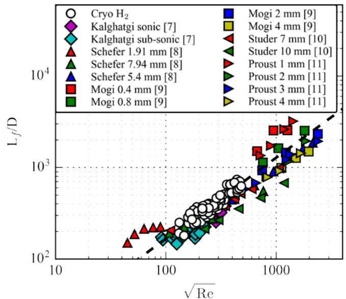
**FIGURE 4.** Variation of flame length as a function of Reynolds number (Re), for the cryogenic hydrogen releases from the current study, along with data from the literature
