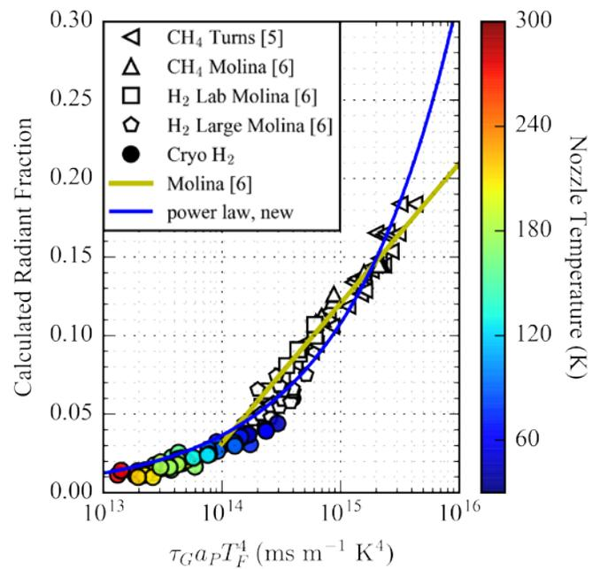
**FIGURE 3.** Radiant fraction from cryogenic hydrogen jet flames and literature data of flames from atmospheric temperature source gases
