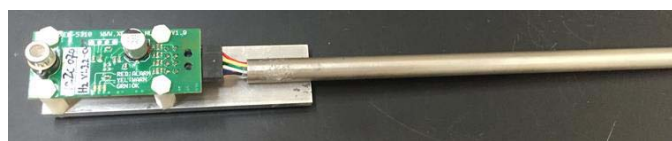
FIGURE 1. Prototype hydrogen probe for FCEV tailpipe exhaust. A ruggedized probe for field use is under development.
