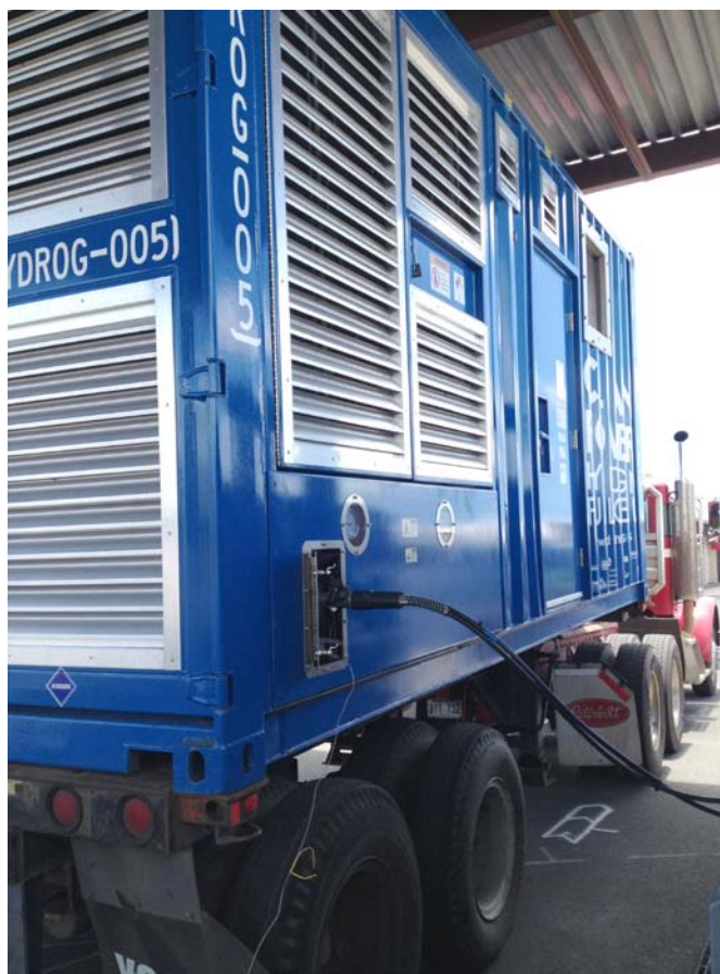
FIGURE 4. The generator was fueled at the Hickam Hydrogen Station (managed by Hawaii Center for Advanced Transportation Technologies and operated by U.S. Hybrid). Here it is being refueled to 350 bar with 49 kg of hydrogen in 18 min.
