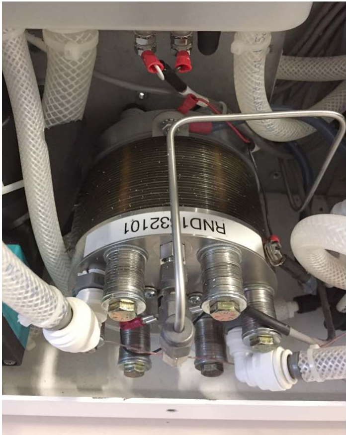
FIGURE 3. Cell stack and system instrumented for thermal measurements
