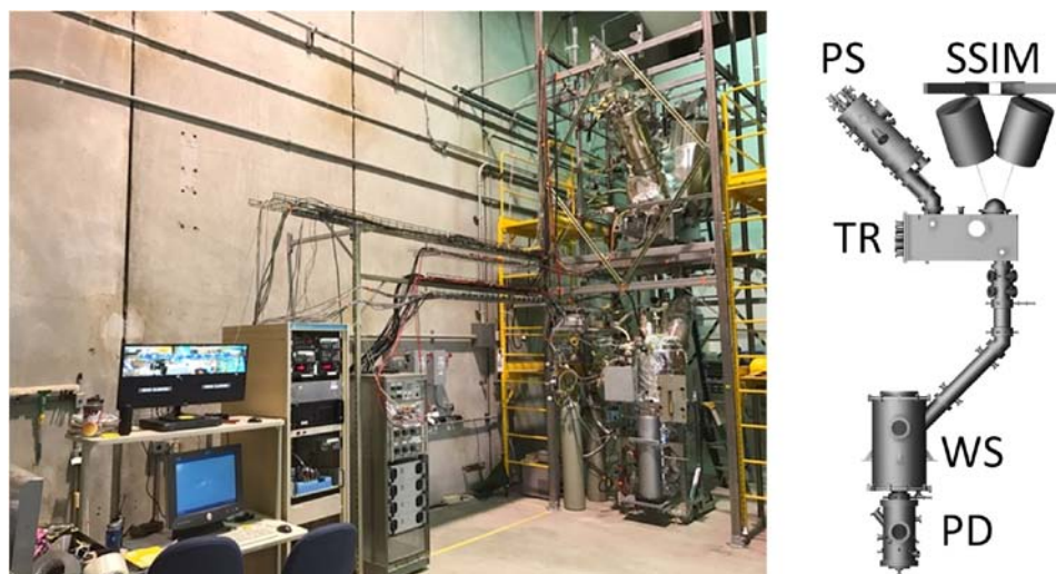
FIGURE 2. Image and schematic of Sandia’s fully assembled and operational CPR 2 . PS = particle source chamber, SSIM = 4-lamp, 20 kW ele solar simulator, TR = thermal reduction chamber, WS = water splitting chamber, and PD = particle drain (see text for details).
