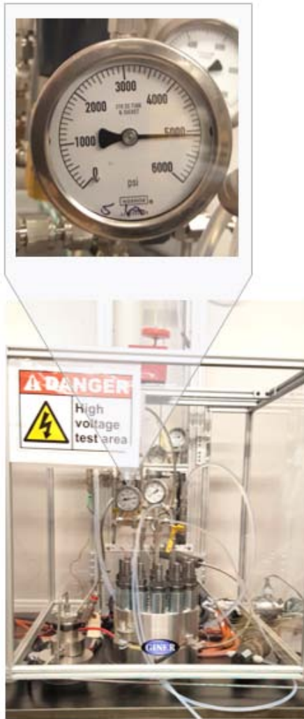
FIGURE 3. EHC stack, 5,000 psi operation
