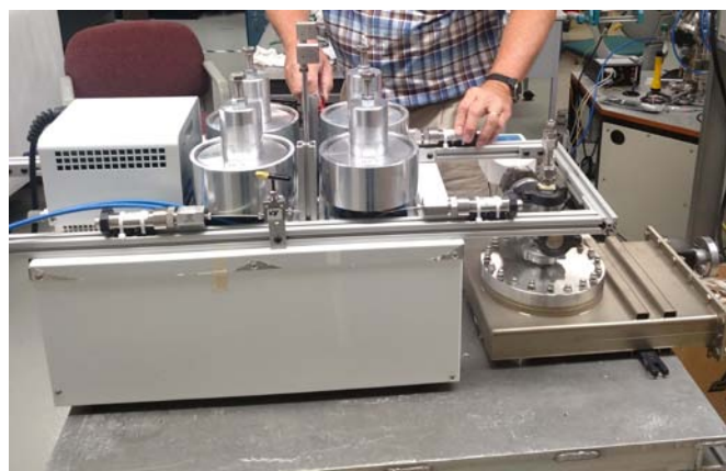
FIGURE 3. Picture of the high pressure Sievert's apparatus designed and assembled by ORNL
