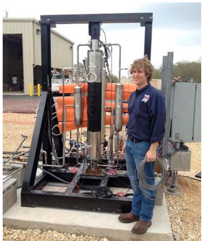
FIGURE 3. Photo of LMRC fully assembled and mounted on the test stand supporting structure
