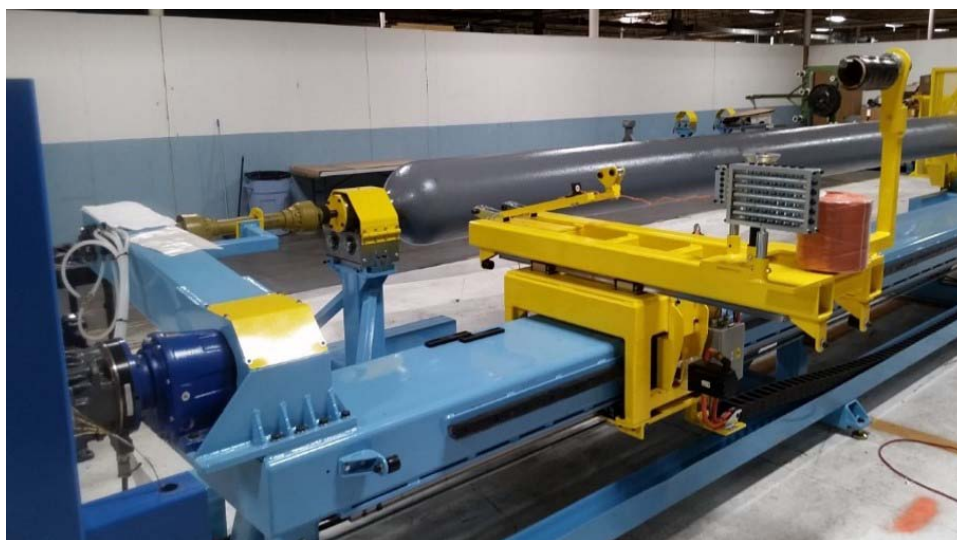
FIGURE 1. Photograph of an 8-axis wire winding machine procured from MVP, Inc., capable of wire winding 9.2 m long liners now installed in WireTough's Bristol, Virginia, manufacturing facility
