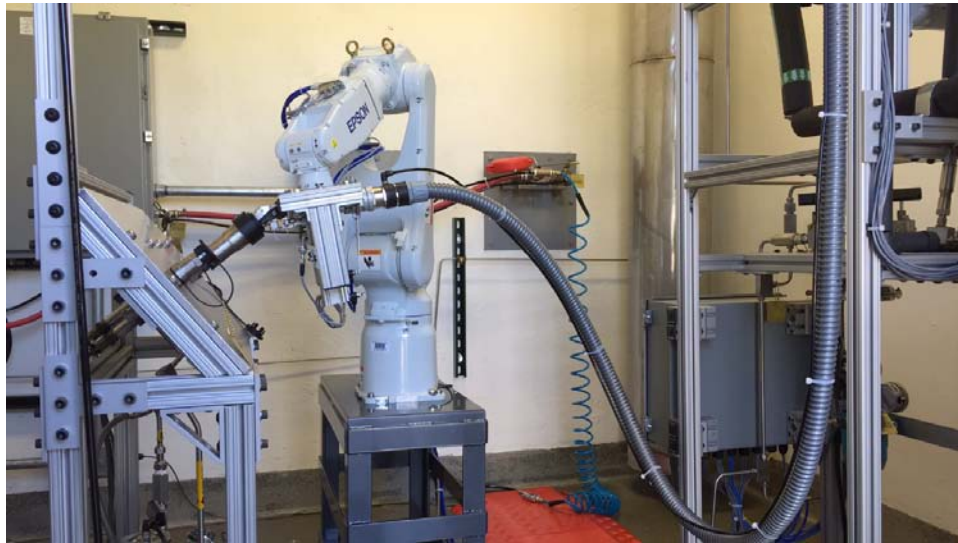
FIGURE 1. Hose reliability test stand
