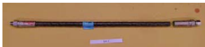
FIGURE 2. NanoSonic hose post hydrostatic burst strength, failure due to fitting slippage
