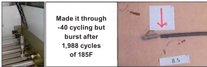
FIGURE 4. NanoSonic H 2 hose post pressure cycle testing at 12,000 psi after 50,000 cycles at -40°C and -1,988 cycles at 85°C; failure shown due to fitting slippage
