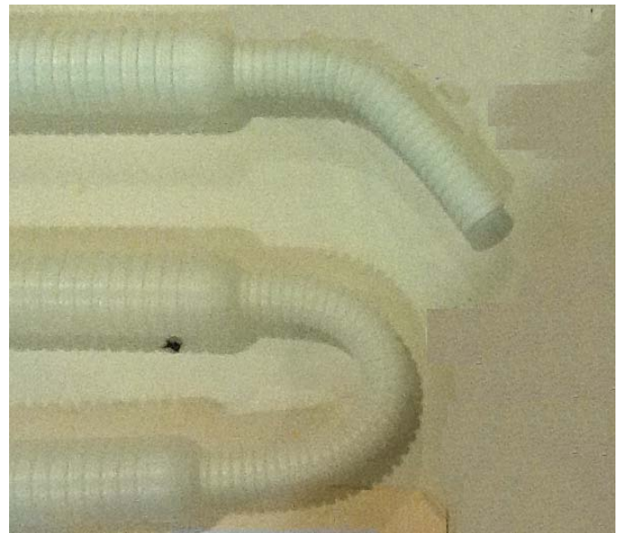
FIGURE 3. Blended EVOH core with greater flexibility
