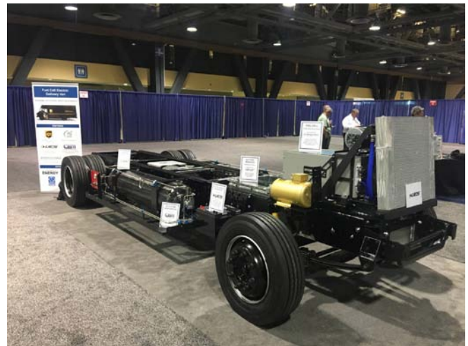
FIGURE 2. The vehicle chassis on the ACT Expo display floor, with primary powertrain components installed
