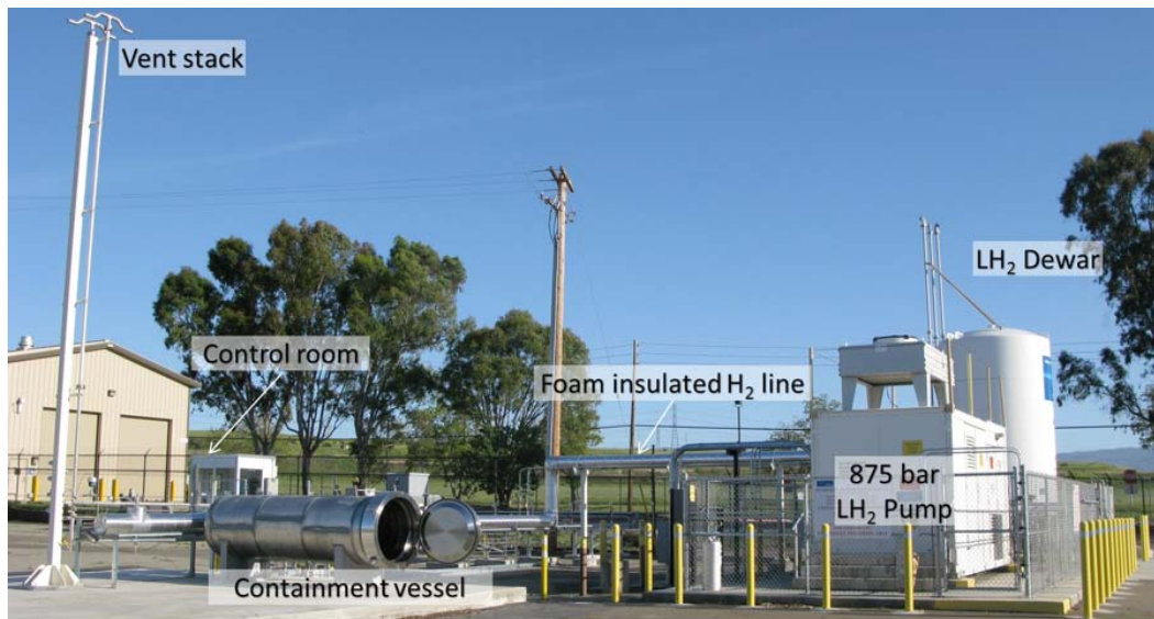
FIGURE 1. Hydrogen Test Facility at LLNL showing the main components
