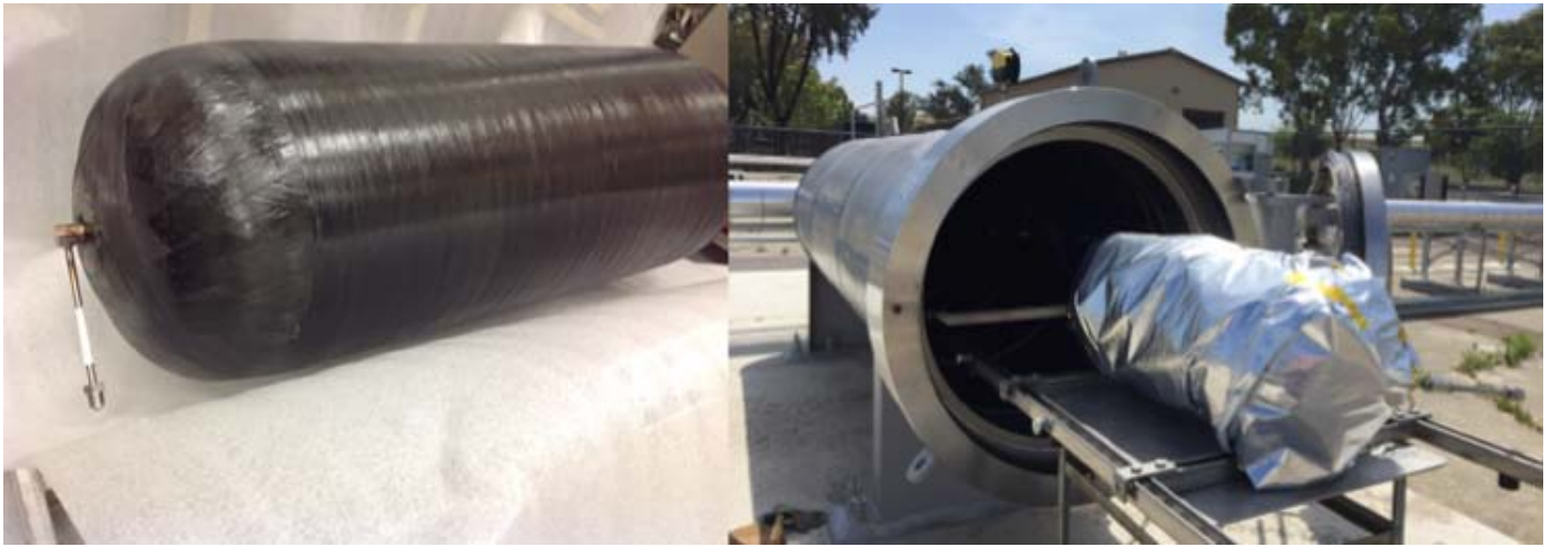
FIGURE 2. Prototype thin-lined experimental pressure vessel (left), and multilayer insulation-wrapped and instrumented prototype vessel being introduced into containment vessel for cycle testing (right)
