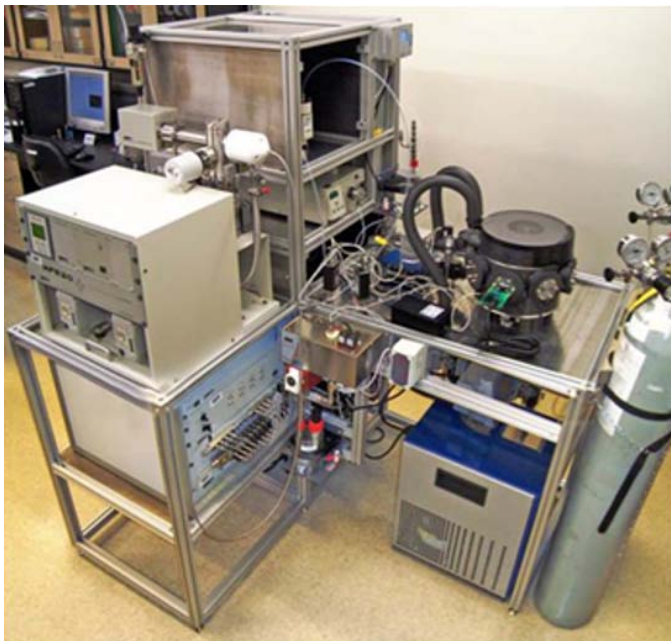
FIGURE 1. The NREL Hydrogen Sensor Test Apparatus
