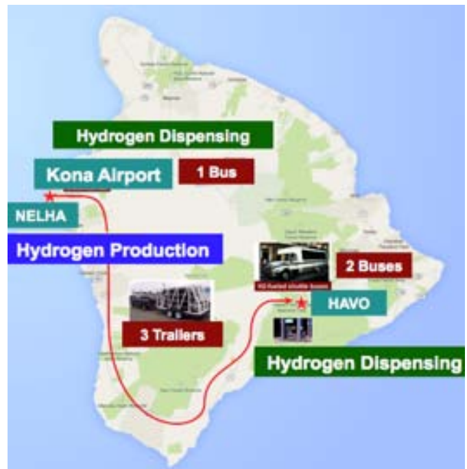
FIGURE 1. Hydrogen production and delivery system
