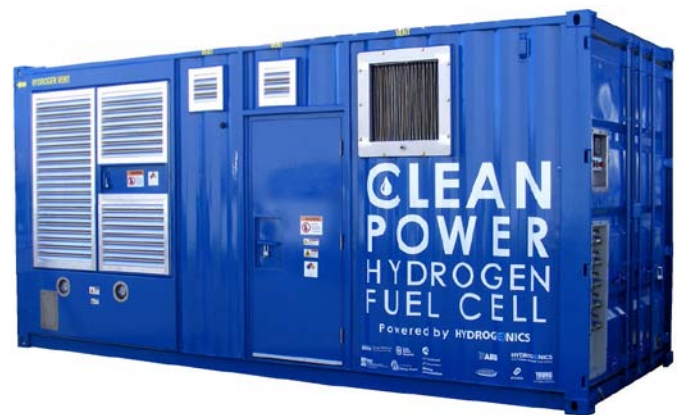
FIGURE 1. The maritime fuel cell generator, with integrated hydrogen storage, PEM fuel cell power generation, and power inverter equipment can power up to 10 reefers with a total rated output of 100 kW at 240 VAC
