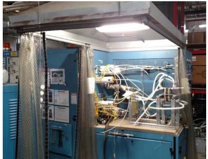
FIGURE 1. Fuel cell stacks at test stand
