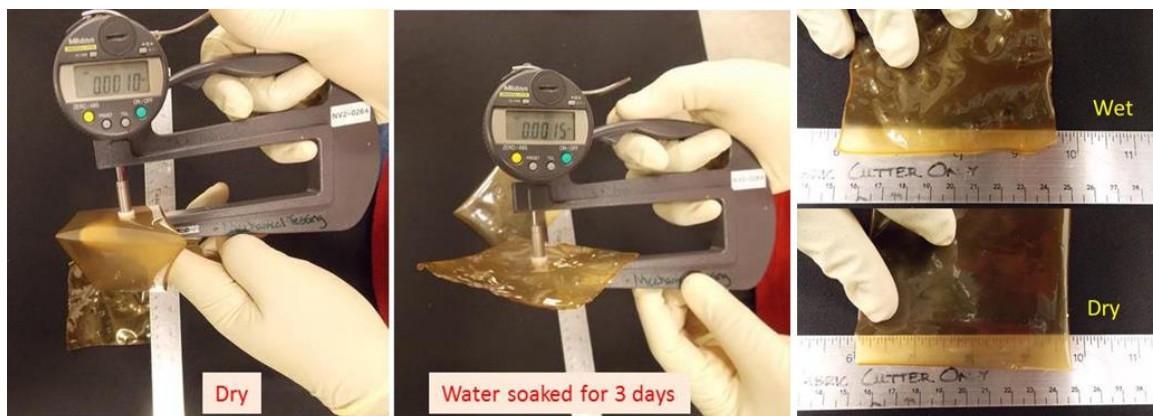
Figure 1. Dimensional stability (low volumetric change) of NanoSonic membranes in dry and wet (hydrated) state
