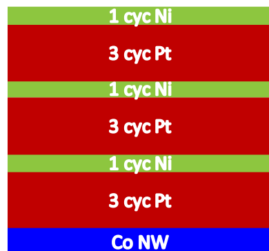
Figure 2. Schematic of Pt-Ni co-deposition onto cobalt nanowires. Microscopy and energy dispersive X-ray spectroscopy of the resulting nanowires, shown with Pt (red), Ni (green), and Co (blue).
