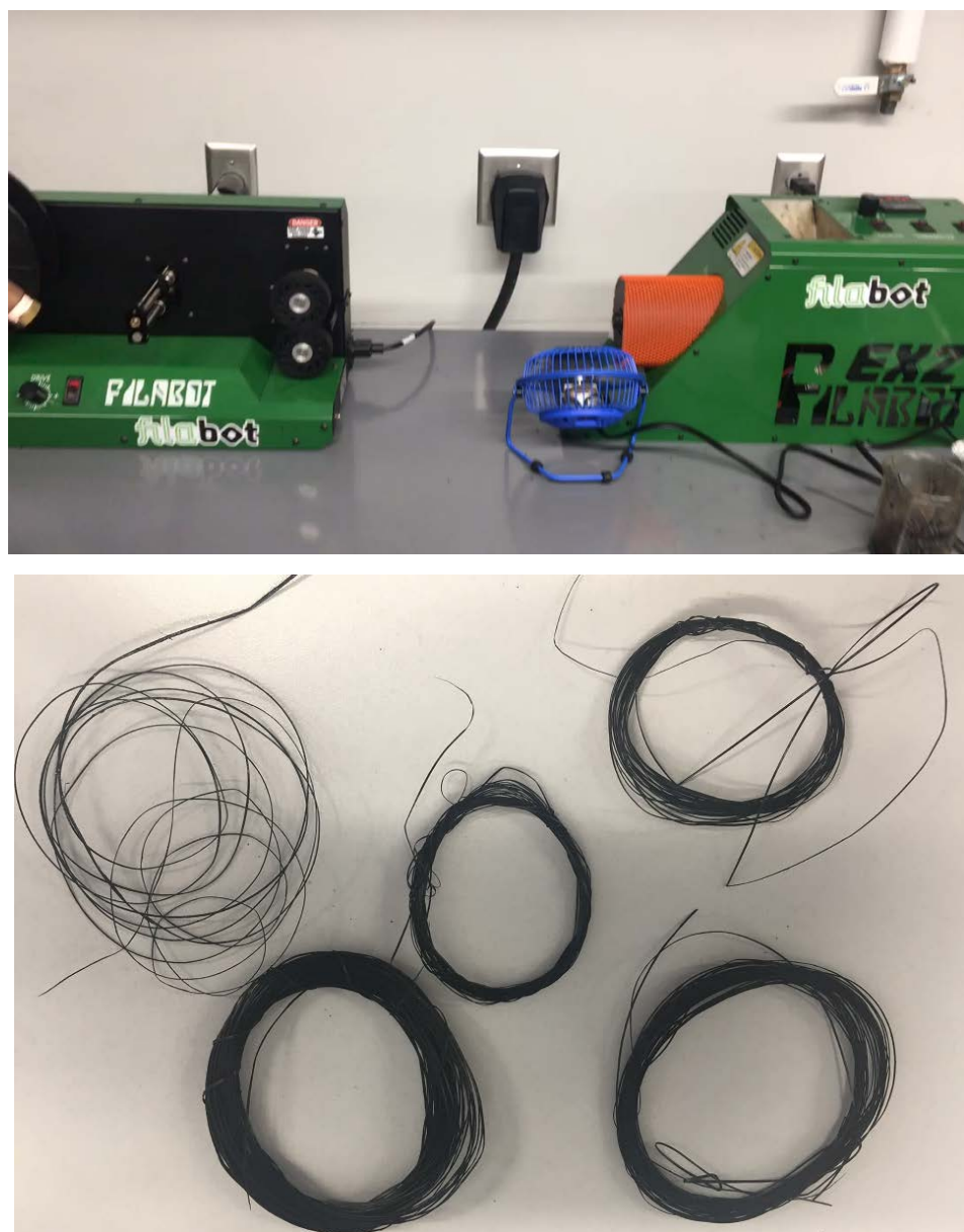
Figure 3. (top) Melt fiber-spinning of a PE-Pitch precursor using a Filabot desktop filament extruder and a spooler with the rotating puller wheels; (bottom) several PE-Pitch fibers prepared by the melt fiber-spinning process
