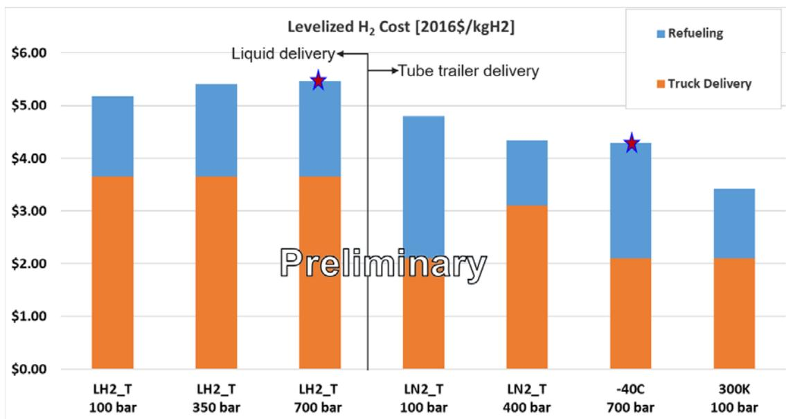
Figure 4. Impact of various FCEV onboard storage P and T requirements on the levelized cost of hydrogen delivery and refueling
