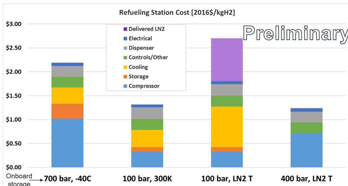
Figure 3. Impact of various FCEV onboard storage P and T requirements on the levelized cost of hydrogen refueling assuming gaseous tube trailer delivery
