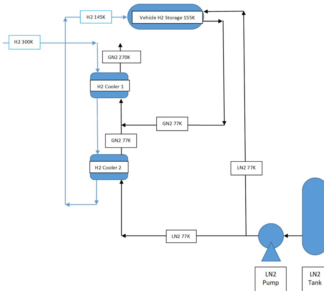
Figure 2. Cooling equipment configuration at hydrogen refueling station that requires LN2 temperature cooling of both hydrogen gas and onboard storage tank
