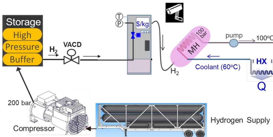
Figure 1. Hydrogen refueling station configuration for a low pressure (100 bar) and near ambient temperature dispensing
