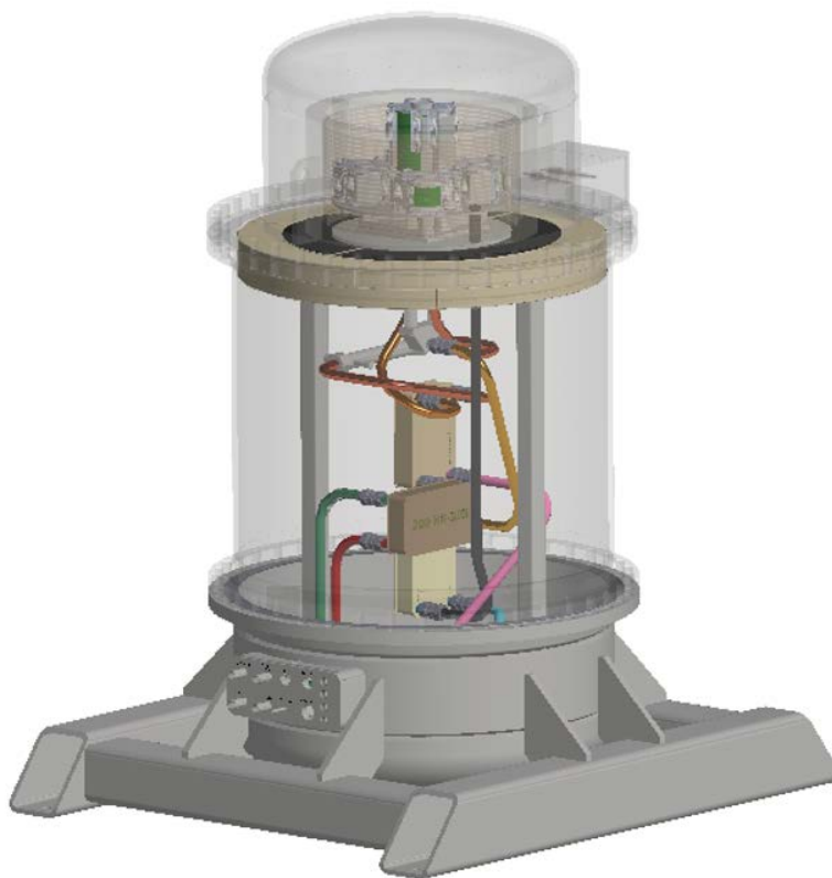
Figure 4. Rendering of the integrated 4 kg H 2 /day pilot demonstration system consisting of a single vessel containing the SOEC module and balance-of-plant equipment
