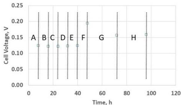
Figure 2. Nafion 117 cell test results during 95-hour operation at elevated temperatures
