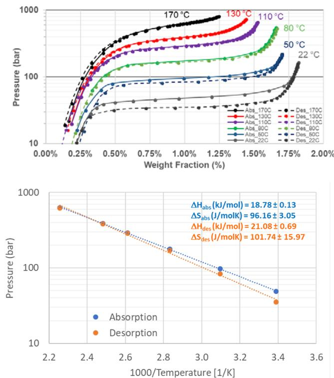
Figure 3. Characterization of MHC candidate HP3 (TiCrMn): (top) absorption and desorption isotherms; (bottom) van't Hoff plot
