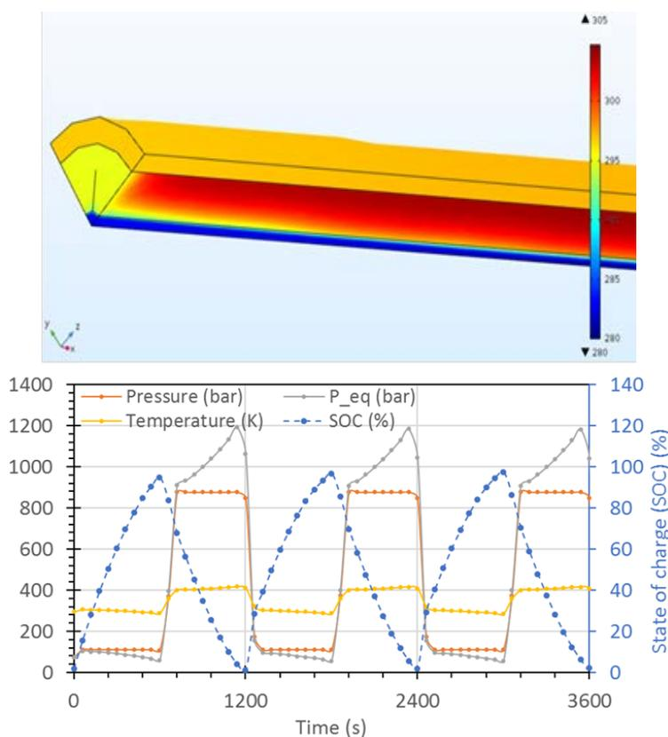
**Figure 4. Detailed MH tank simulation: (top) temperature profile—charging cycle at 150 s; (bottom) pressure, temperature, and state of charge plots for three 20-minute cycles**
