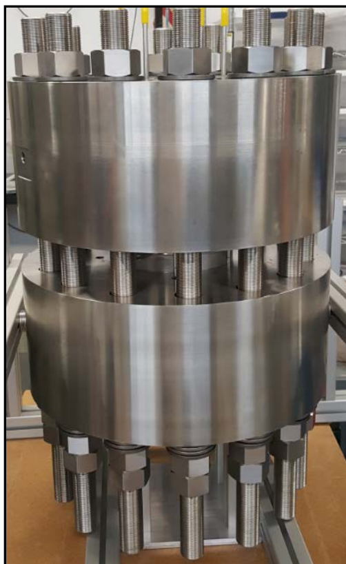
Figure 4. 875 bar EHC stack (50 cm 2 )
