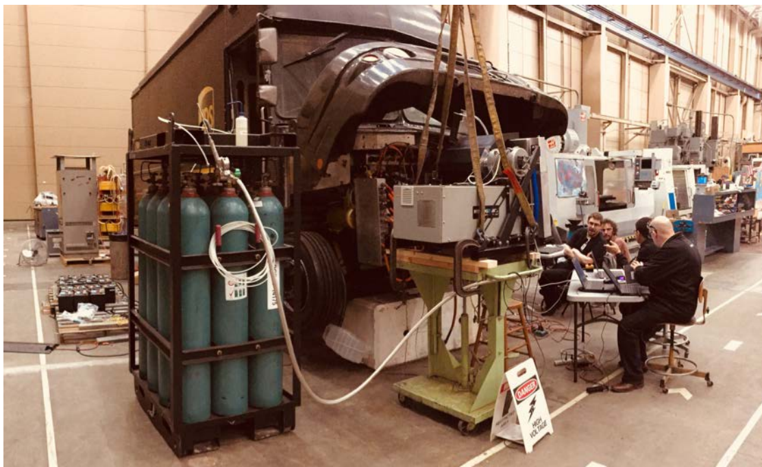
Figure 1. Hydrogenics, Unique Electric Solutions, and UT-CEM monitoring the fuel cell power system during bench tests
